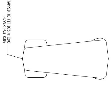
FINISH: HOT DIP GALVANIZED PER ASTM A153
